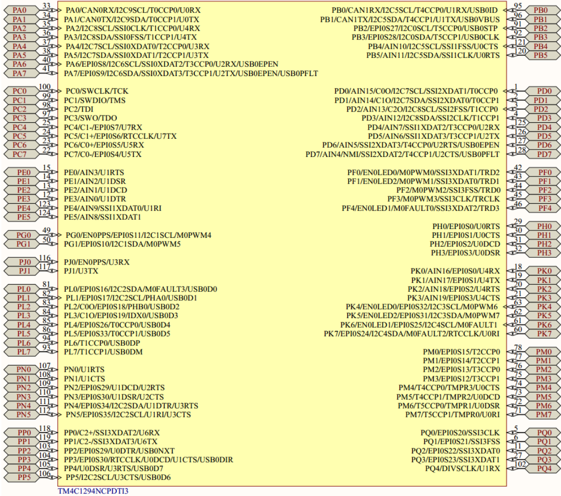
Figure 6.10: Layout of the majority of the TM4C1294NCPDT pins
